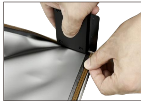
Use scraper tool provided to press the screen into the frame.
